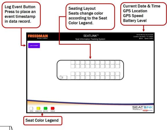
OPEN: This seat is unoccupied and the belt is not buckled.
