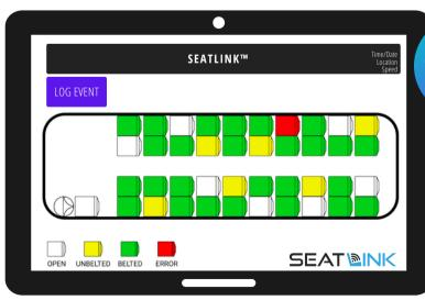
System includes one (1) head unit which records, stores and displays passenger occupancy and seat belt status.
