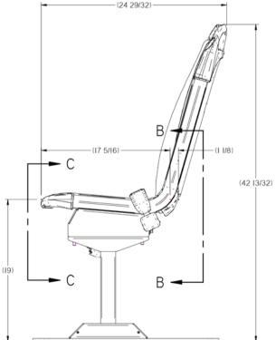
The CitiPro 3PT is manufactured with custom formed aluminum extrusions for superior strength and significant weight savings. The seat and back panels are made from injection molded plastic for comfort, weight and durability. Meets FMVSS 207/210. White Book and Docket 90 compliant.
